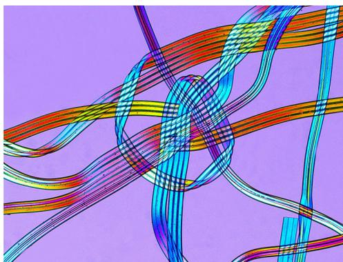
Figure 4.3: Spandex fibers under an optical microscope
